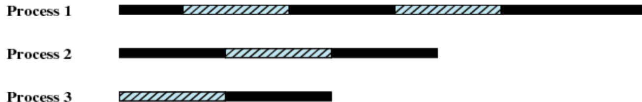
(b) Interleaving and overlapping (multiprocessing; two processors)
